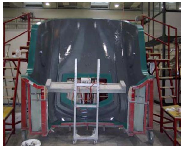
Fig.10. Applying and hardening of the gel coat
